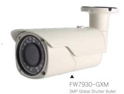
**FW7930-GXM** is a high quality IR bullet IP camera which is equipped with 3.19MP(effective pixel) Global Shutter CMOS image Sensor. With the highest sensitivity sensor, it is especially superior in low light condition. As it supports simultaneous H.265, H.264 and MJPEG Video Compression, less network bandwidth and storage space required. It also delivers high quality video image at 30 fps @ 3MP (2048X1536) in progressive mode,
